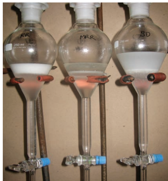
Figure 2. Phase separation of the first separation step during extraction of PLs from BMP. Left, method of Rombaut et al.; 16 middle, own modified method with addition of \text{CaCl}_2 ; and right, B&D method.
